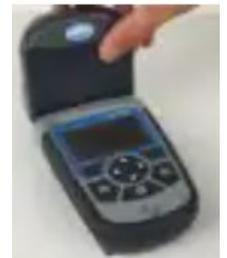
20. Press the SELECT button to display the chlorine value in the 10 ml sample bottle.
