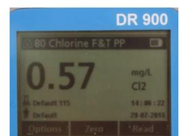
21. Compare the reading on the DR900 to the reading recorded in step 6 from the HACH CL17 SC.
