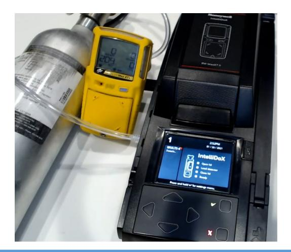
• Ensure the detector is powered up and showing gas readings before docking
