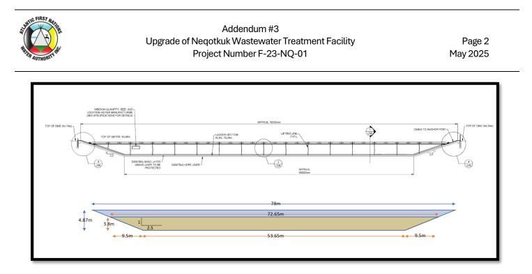
**Answer:** The top water elevation (of 83.08 m) and bottom elevation (of 79.28 m) are correct. The top width is approximately 78.0 m. Please revise the bottom width to 45.0 m and update the side slopes to 3H:1V.
