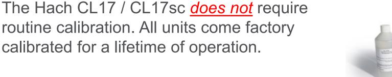
The CL17sc calibration curve is set at the factory for performance to specifications. User adjustment of the factory calibration curve is only recommended in two instances: if required by a regulatory agency for compliance reporting purposes or if a large repair of the analyzer is done.
