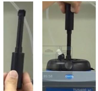
23. Reinstall the process head on the cell cover.
