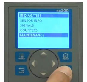
10. Scroll down to VIAL CLEANING with the DOWN ARROW key.
