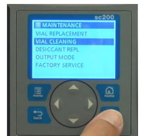
12. The next screen that appears instructs the operator to SWITCH OFF THE INFLUENT FLOW AND OPEN THE PROCESS HEAD.
