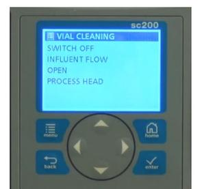
13. Close off the sample flow into the analyzer.
