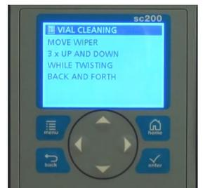
21. Insert the wiper into the flow cell and go up and down three times in a twisting motion.
