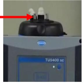
15. Place the process head in the maintenance rack.
