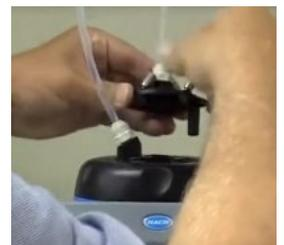
24. Turn on the influent flow returning the influent flow to the flow cell.
