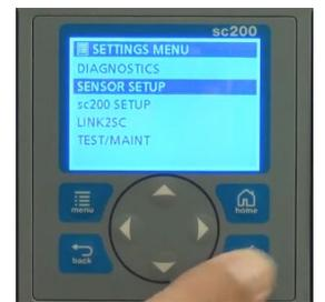
6. Scroll down to DIAG/TEST with the DOWN ARROW key.
