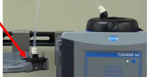
16. Remove the cell cover and empty any water in the flow cell to prevent any water spilling on the top of the instrument.
