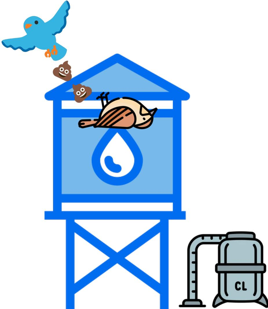
Reservoirs provide contact time for chlorine to disinfect and inactivate bacteria and viruses.
