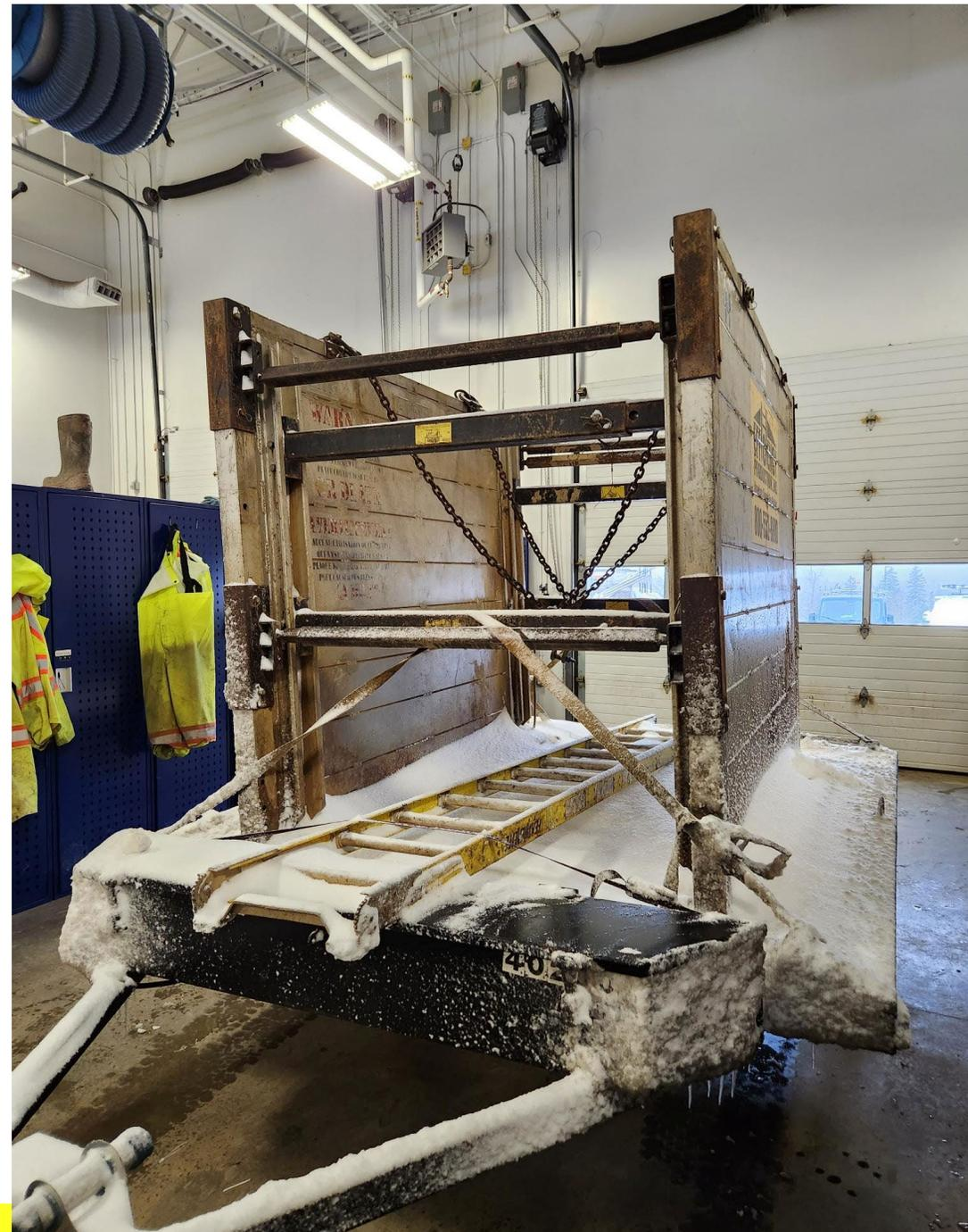
Another method to make trenches safe is shoring. This is the use of temporary props or supports that are used in conjunction with planks, sheeting or other materials that are propped against the walls to support them. This method can be much more time consuming, and if not done correctly is more prone to failure.
